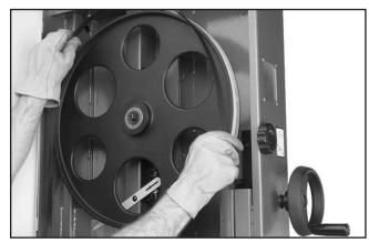
Figure 48. Placing blade on the wheels.
